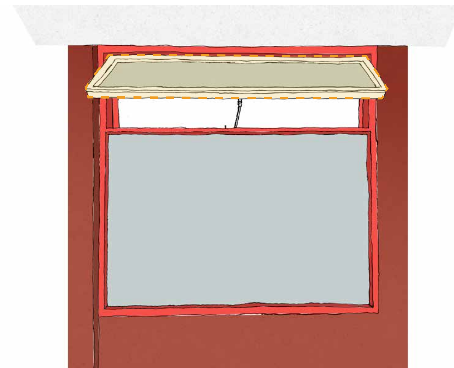
Option 03: Primary window frame repaired, and opening light replaced with hardwood frame
