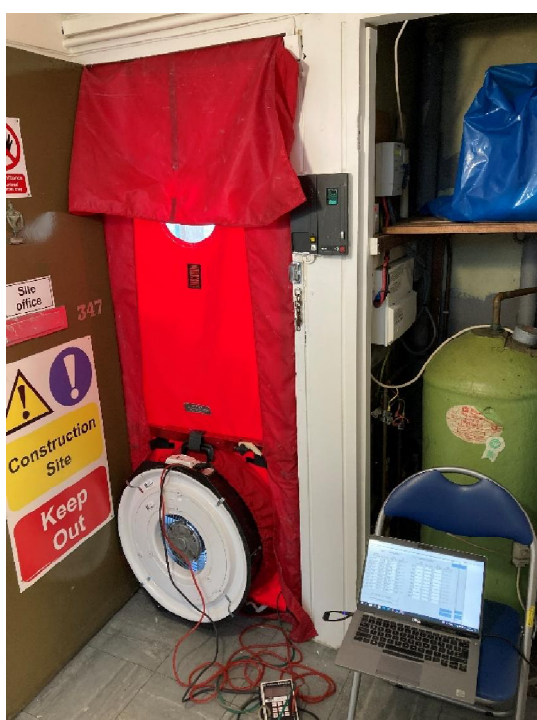
Figure 2: Test set-up showing the blower door mounted in the front door.
