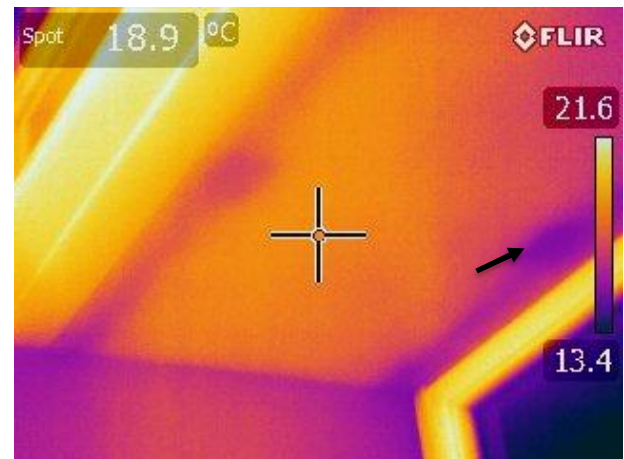
Figure 15: Thermal Image - front window reveal - heat loss highlighted Location THL7
